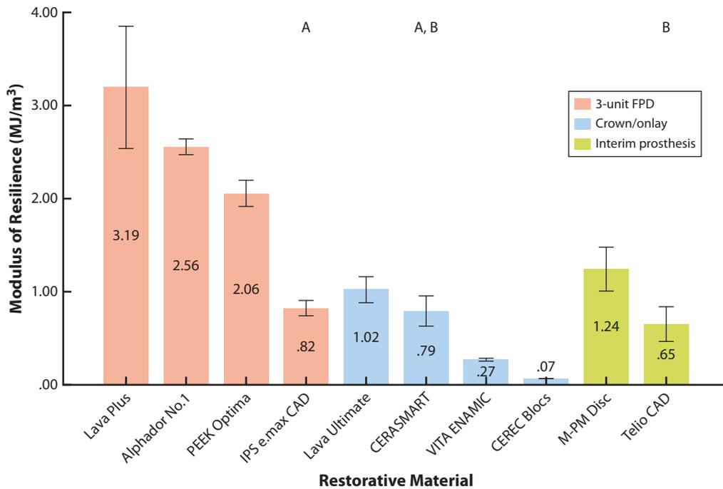
**Figure 4.** Mean modulus of resilience (MJ/m<sup>3</sup>) with error bars representing standard deviation. Identical uppercase letters denote no significant differences among groups ( $P>.05$ ).
