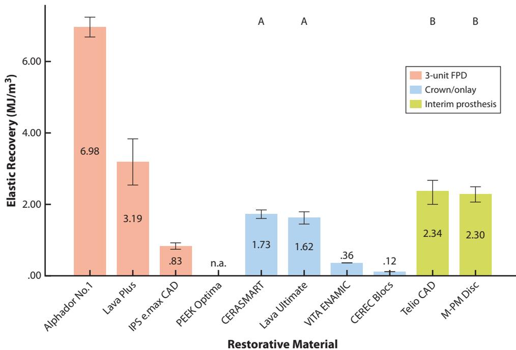
**Figure 5.** Mean elastic recovery (MJ/m<sup>3</sup>) with error bars representing standard deviation. Identical uppercase letters denote no significant differences among groups ( $P>.05$ ). n.a., not available.
