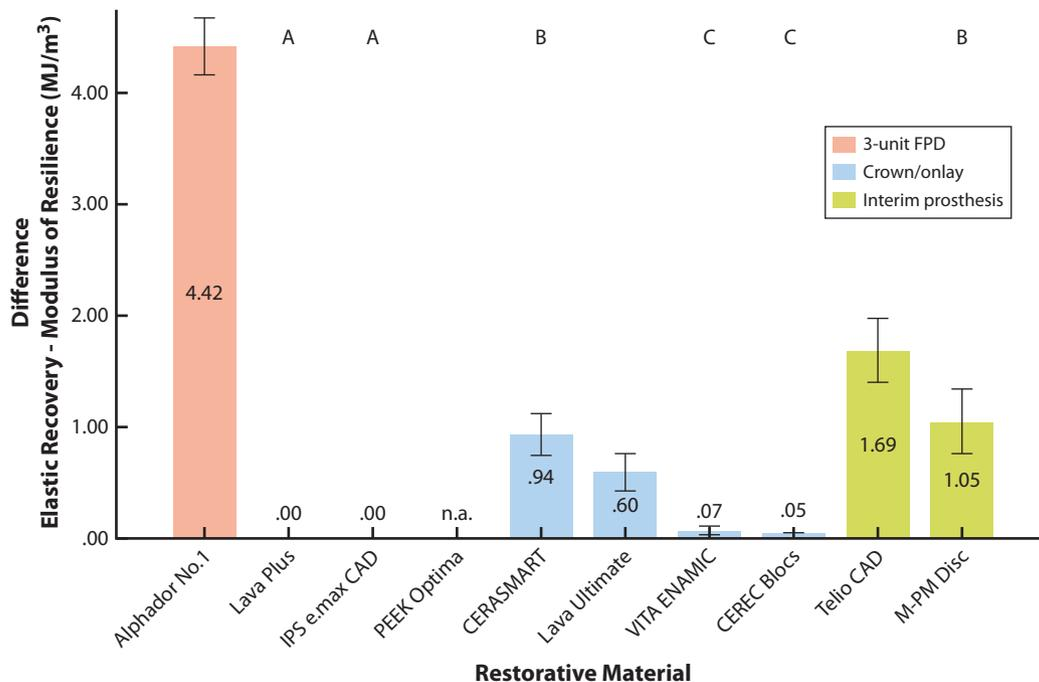
**Figure 6.** Mean difference between elastic recovery and modulus of resilience (MJ/m<sup>3</sup>) with error bars representing standard deviation. Identical uppercase letters denote no significant differences among groups ( $P > .05$ ). n.a., not available.
