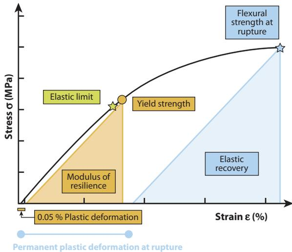
**Figure 1.** Stress-strain curve exemplifies elastic energy absorption during specimen bending. Areas of triangles represent strain energy density for elastic energy dissipation without or with permanent plastic deformation.
