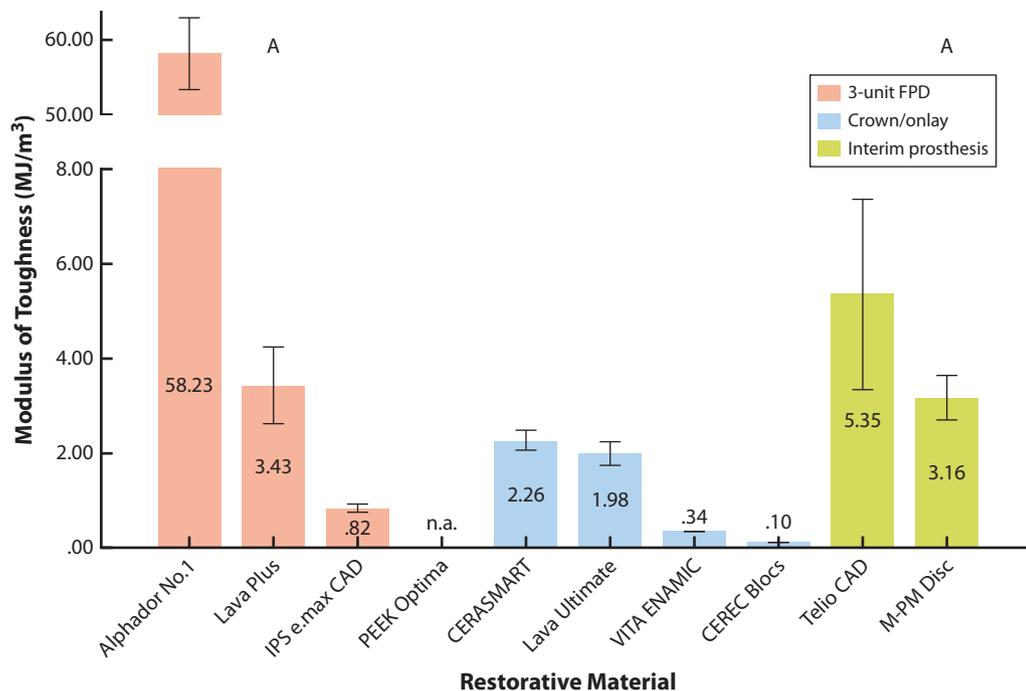
**Figure 3.** Mean modulus of toughness (MJ/m<sup>3</sup>) with error bars representing standard deviation. Identical uppercase letters denote no significant differences among groups ( $P>.05$ ) n.a., not available.
