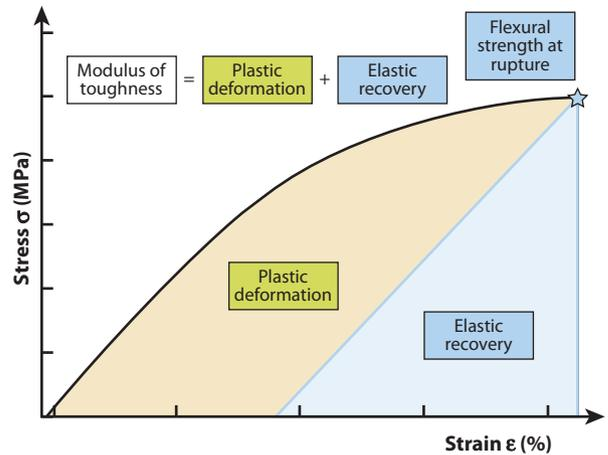
**Figure 2.** Stress-strain curve exemplifies combination of elastic with plastic energy absorption during specimen bending. Area up to rupture represents total strain energy density for energy dissipation (modulus of toughness).
